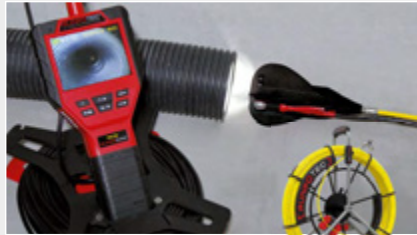
Pipe inspection for large pipe diameters
