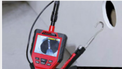
Cavity wall inspection, locating and capturing
