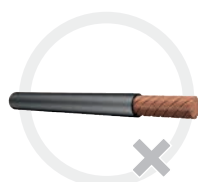
Excessively twisted individual wires
