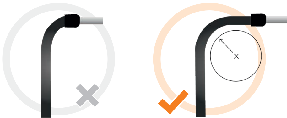
Risk of breakage due to overload
