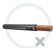
Damaged conductor insulation
