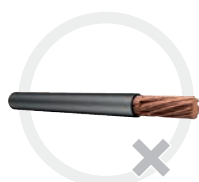
Damaged or cut-off individual wires
