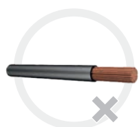
Too less twisted single wires
