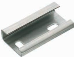
TS 32 mm according to EN 60715 (s = 1.5 mm)
