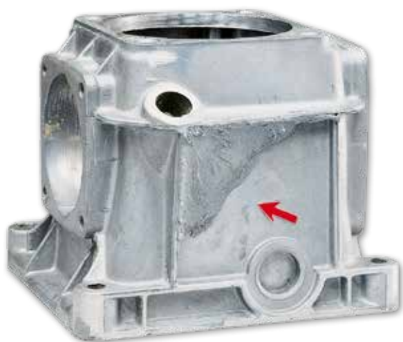
Reconditioning of an aluminium housing
