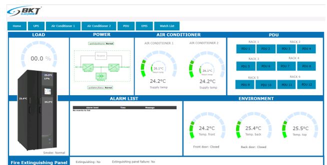
The ability to visualize device statuses with external software, such as BKT SM4DC, using SNMP protocol.
