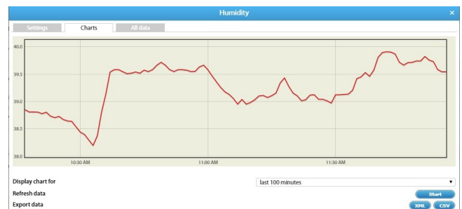
Displaying a limited (100s, 100min, 100h, 100days) log of sensor measurements on graph.
