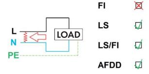
If there is a failure between L and PE, a RCCB, a RCBO and an AFDD can recognized it and switch of.
