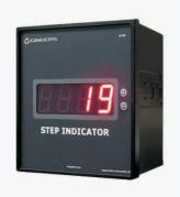
SI4080 and SI4100 are digital measuring, fully programmable panel instruments from series 4080 and 4100. SI4080/4100 shows the current position of the tap changer of the high-voltage transformer in electrical substations. These meters are part of tap changer-motor drive equipment. The position of the tap changer can be read either analogue (by resistor matrix) or digital (BIN or BCD input). SI4080/4100 are designed to be mounted on boards in control rooms in electrical substations.
