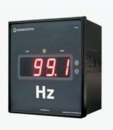
F4080 and F4100 are digital, fully programmable panel instruments from series 4080 and 4100. F4080/F4100 devices are used for frequency measurement 50/60Hz in electrical substations and power plants. They are powered by the measured AC voltage. F4080/4100 have potential-free contacts for remote signalization if measured frequency goes out of certain specified range (option " $\mathbf{R}$ "). F4080/4100 are designed to be mounted on boards in control rooms in electrical substations.
