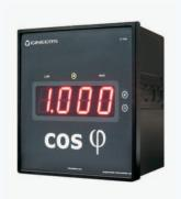
CF4080 and CF4100 are digital measuring, fully programmable panel instruments from series 4080 and 4100. CF4080/4100 measure signed value of cosine of phase angle between their voltage and current inputs. CF4080/4100 are designed to be mounted on boards in control rooms in electrical substations.
